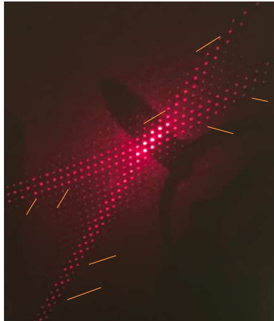
Figure 2. Patterns: rotating grating CCW around X by 45^\circ , CW around Y axis by 45^\circ and CCW around Z axis by 70^\circ
