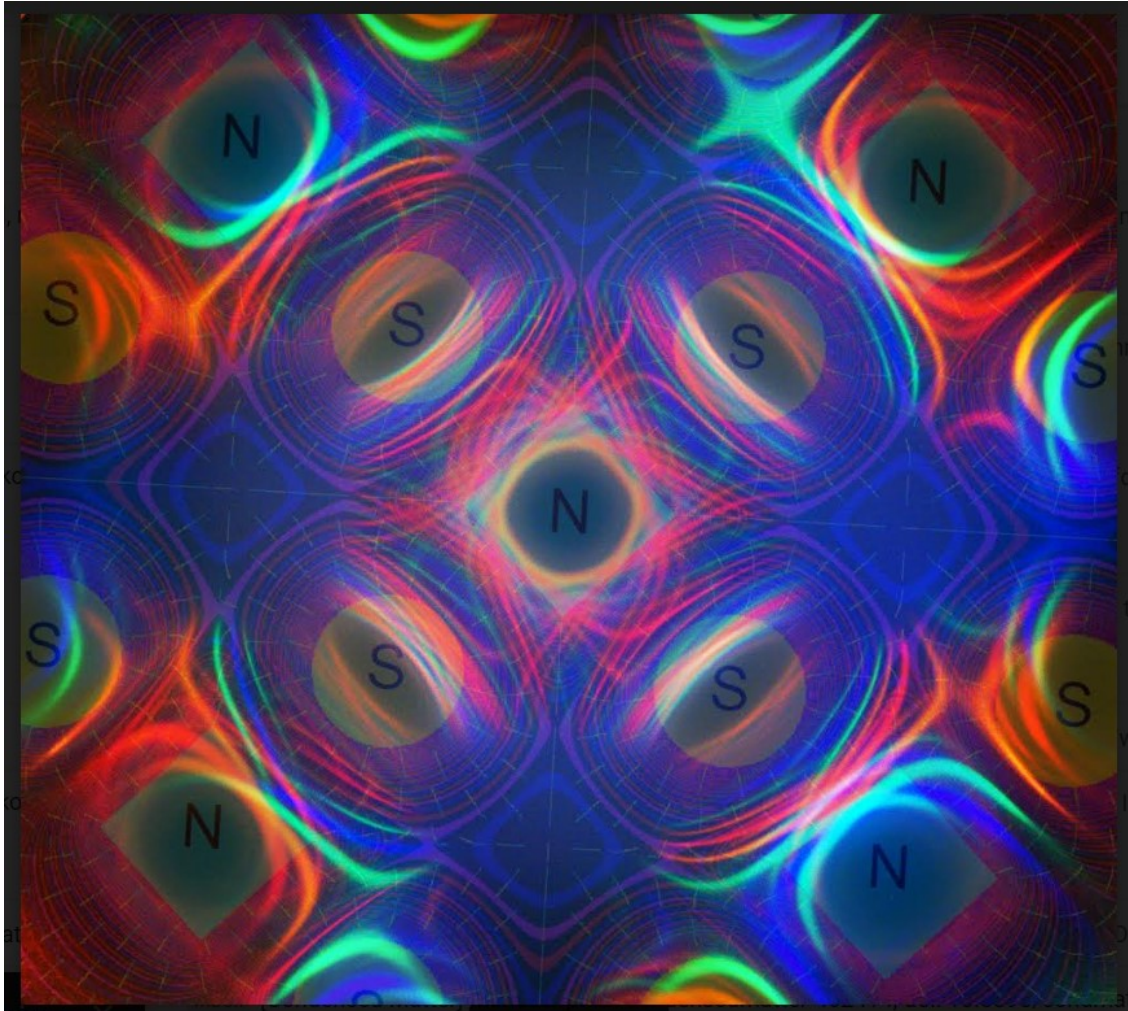
Figure 4.3 –Another array of magnets superposed on the simulation of the magnetic field and isopotentials.
