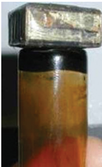
Fig. 1. Photographs of a ferrofluid holding its weight on the inverted vial. On removal of magnetic field, it flows like water.
