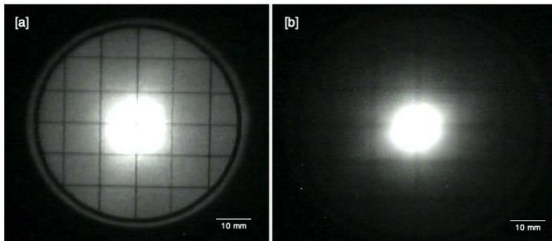
**Fig. 8.** Beam profiler camera images of Plano-concave lens. [a] at 70 mm and [b] 30 mm from target.
