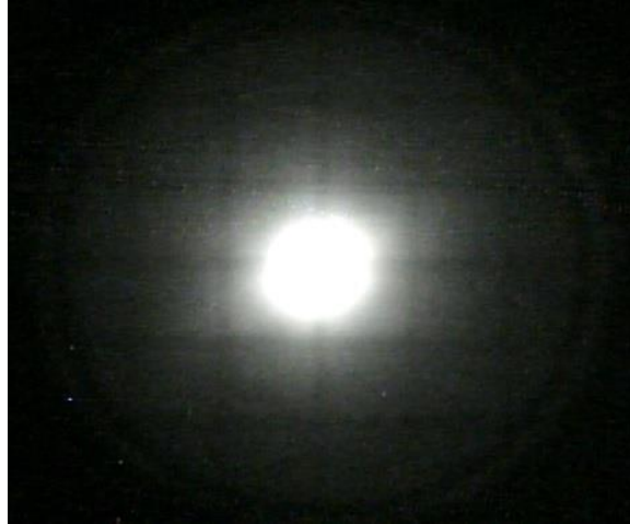
Figure 8c. Circular pattern image of Plano-concave lens 35 mm from first target using beam profile camera.
