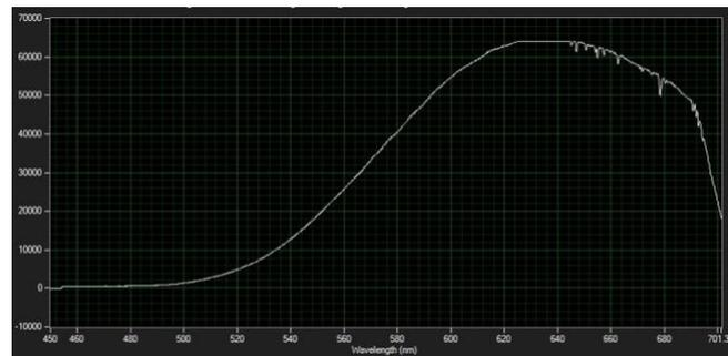
**Fig. 2.** Absorption spectrograph Halogen light transmitted through the 30 micron thin-film.
