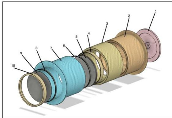
**Fig. 4.** Helmholtz coil insert exploded view with numbered parts.
