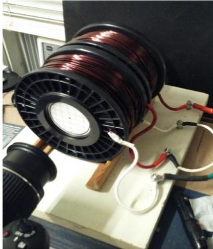
**Fig. 3.** Helmholtz coil. Insert, target, camera and connections visible.
