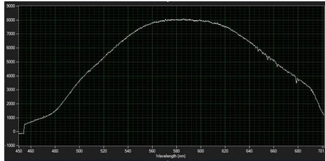
**Fig. 1.** Absorption spectrum of Halogen light for reference.
