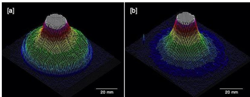
**Fig. 9.** Beam profiles of Plano-concave lens. [a] at 70 mm and [b] at 30 mm from target.
