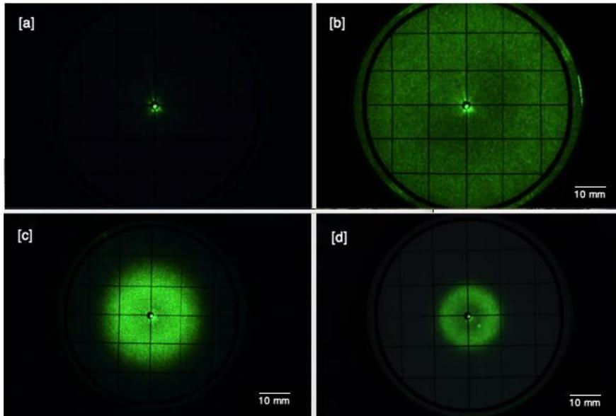
**Fig. 5.** Scattering patterns. No EM: [a] 70 mm from target. With EM: [b] 70 mm, [c] 30 mm, [d] 20 mm distance from target.
